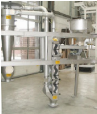
ZZ-Separator SepK12/120-2 Processing of dried vegetables. Removal of foreign substances such as hair, dust, paper, fibres
