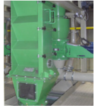
Hybrid-Separator SepHY 10/120-2 Separation of textile from rubber powder
